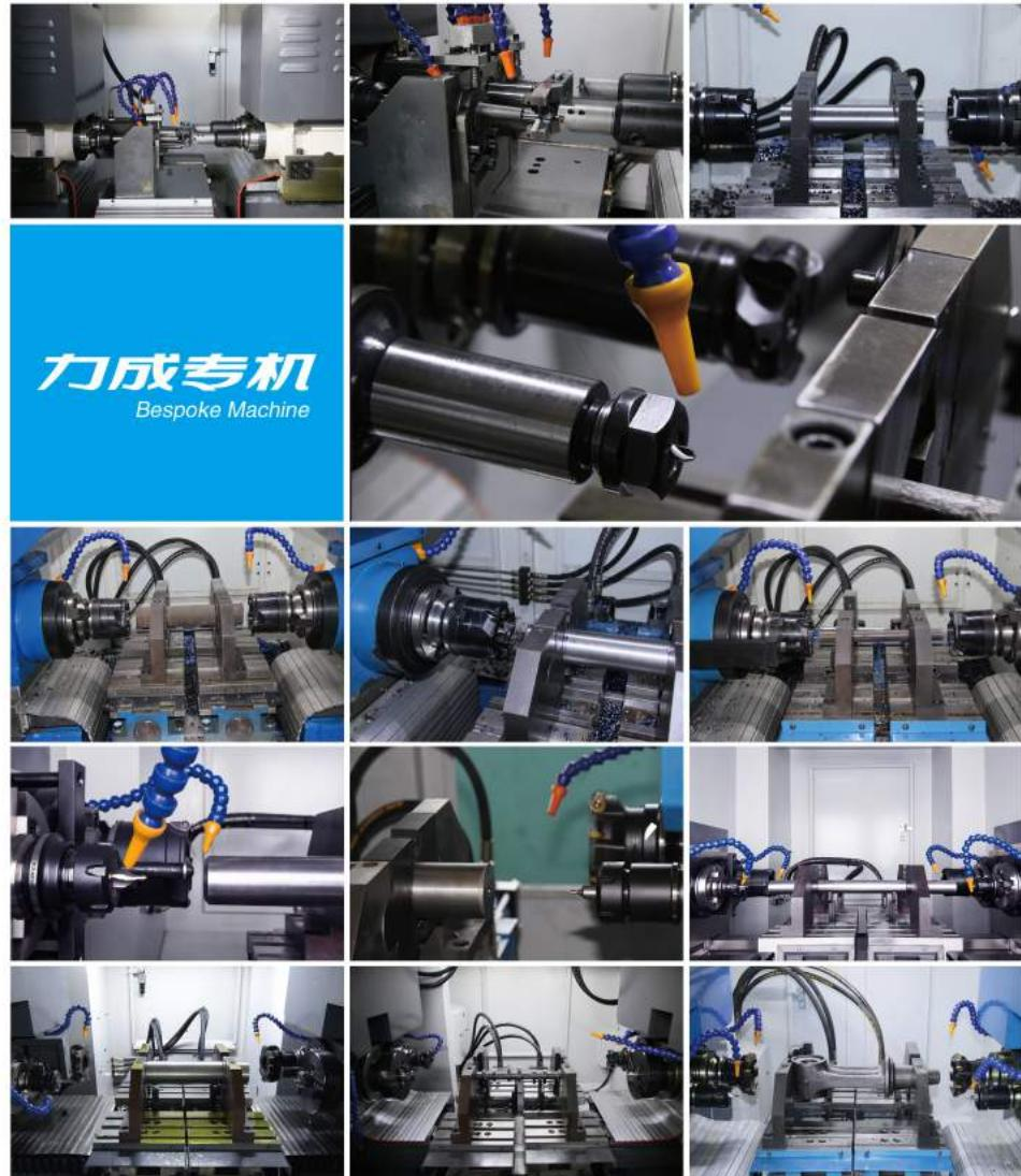
铣端面钻中心孔机床 Facing and centering machine
