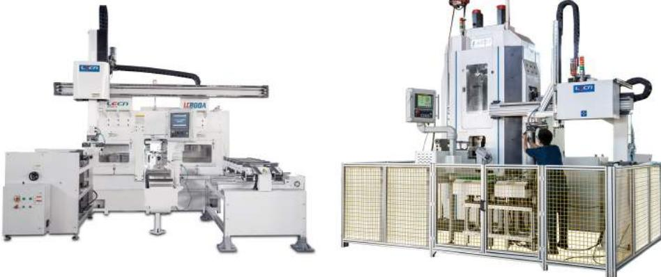
Rolling machine+Truss robot
