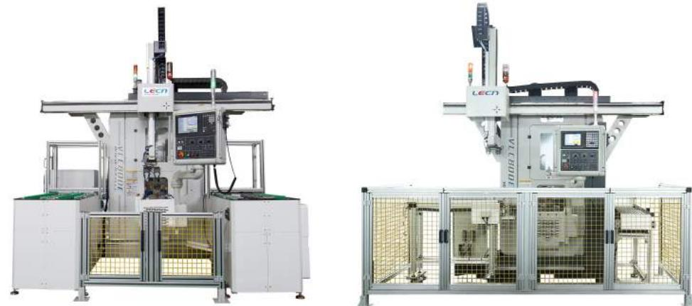
Rolling machine+Truss robot
